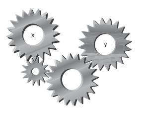
If cog X turns in a clockwise direction, which way will cog Y turn?
