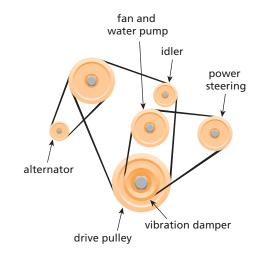
If the drive pulley in a work van engine turns in a clockwise direction, in which direction will the alternator turn?
